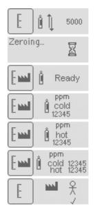
\* Fill an empty (uncontaminated) sample bag with 5000 ppm Helium gas before starting the calibration procedure. Also remove the outer grey probe from the GasCheck G.
