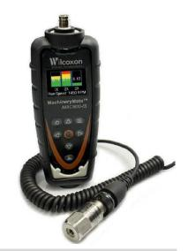
Wilcoxon's handheld MAC800-IS vibration meter analyzes and displays vibration signals, helping users identify machine faults before they impact operations or lead to failure. The meter comes with built-in band filters for unbalance, misalignment and looseness, and its low frequency range allows readings on machinery running at speeds as slow as 120 RPM. The meter is IECEx/ATEX and SGS certified intrinsically safe for use in Class 1 Zone 1 hazardous locations.
