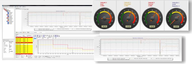
In spectral charts, the user can observe in a more detailed view every feature of each component in a vibration trend, and the application also offers tools for fast and user-friendly automatic analysis.
